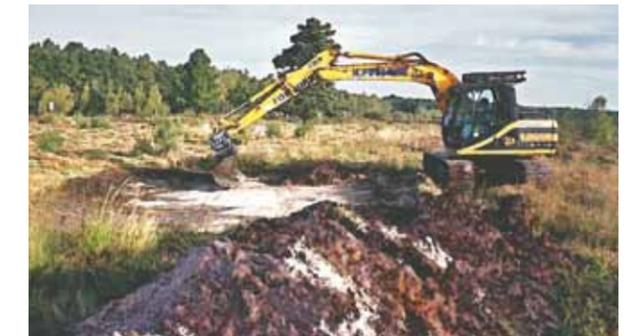
Machinery such as a 13 tonne, tracked, 360° excavator is suitable for creating natterjack scrapes (John Buckley)
